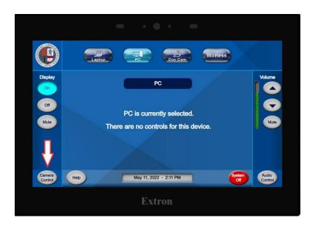
6. The camera can be adjusted to the proper position here. Four presets may also be saved if needed. Press **Close** to return to the main menu after adjustment.
